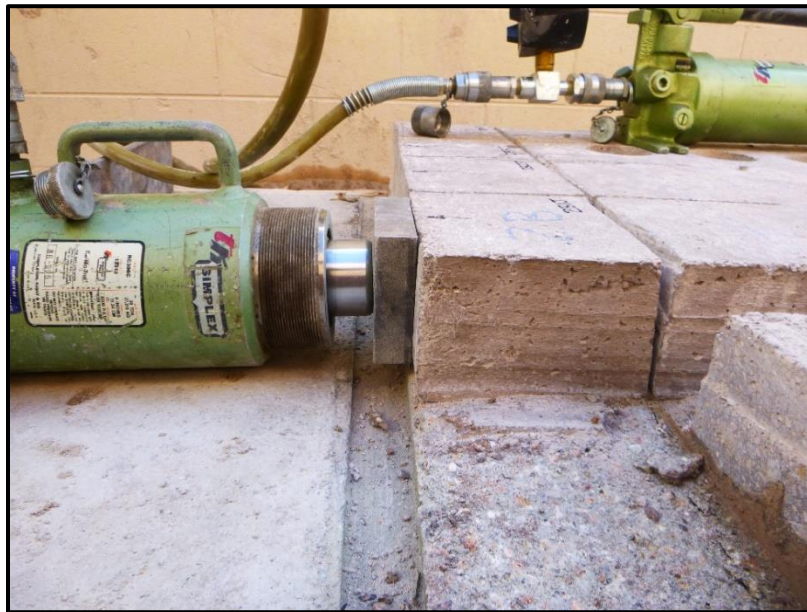
Figure 2-5 – Block specimen undergoing jacking test
