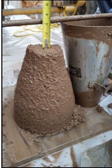
Figure 3-10 – Example slump cone test on overlay concrete (note integral color)
