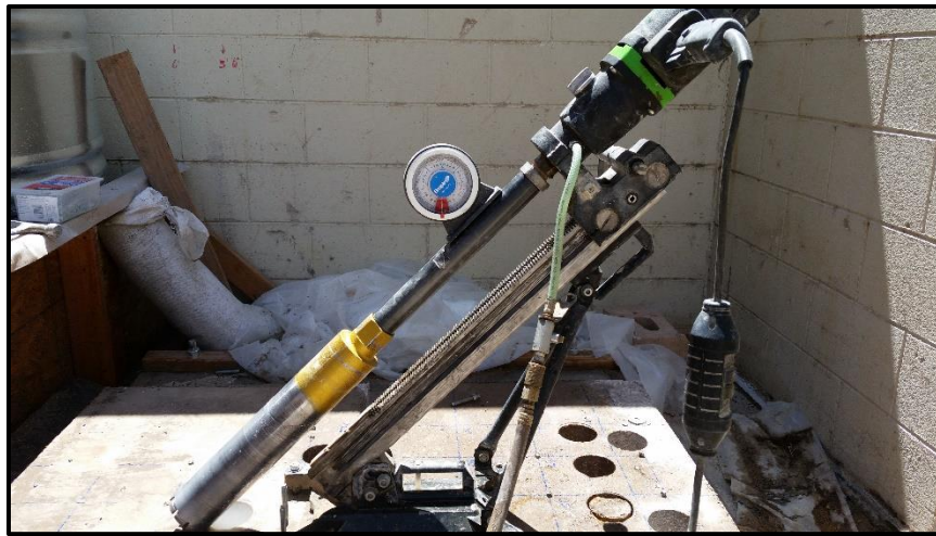
Figure 3-17 – Checking the slant angle with an inclinometer prior to coring for a slant shear specimen
