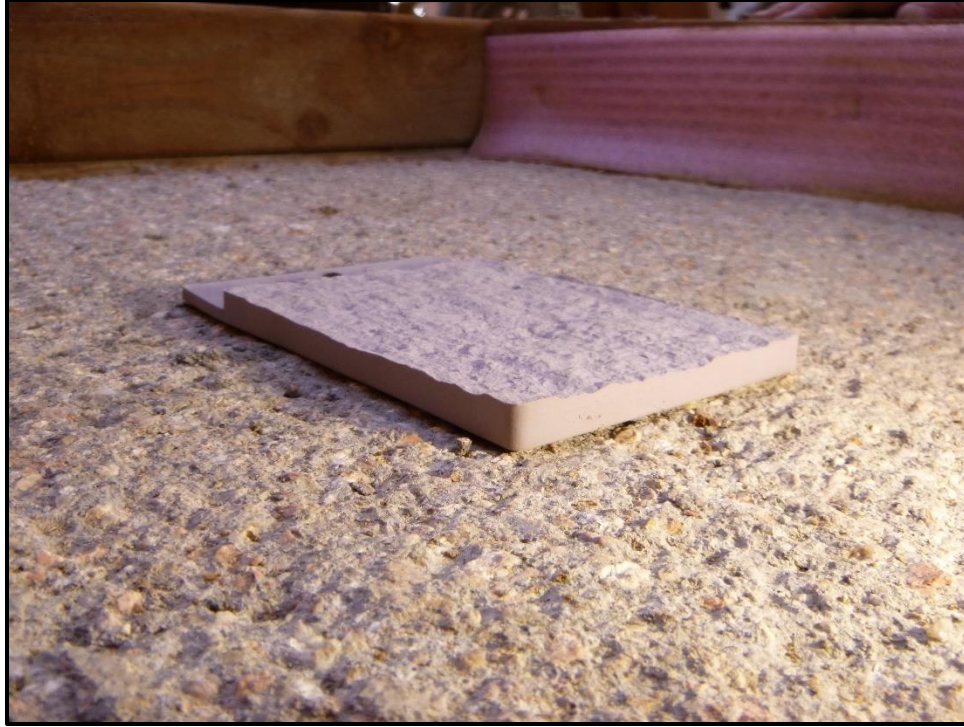
Figure 3-3 – Finished profile compared with ICRI CSP 6 example.
