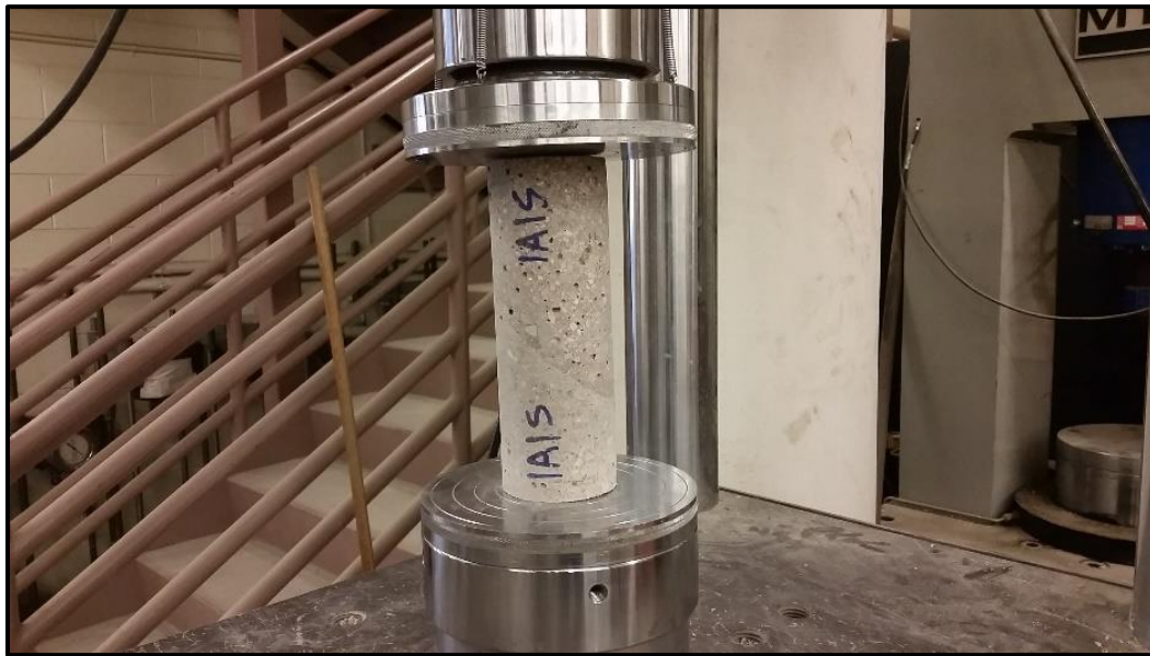
Figure 2-3 – Preparing to test slant shear sample on compression machine. Note difference in concrete color indicating the slanting bond surface
