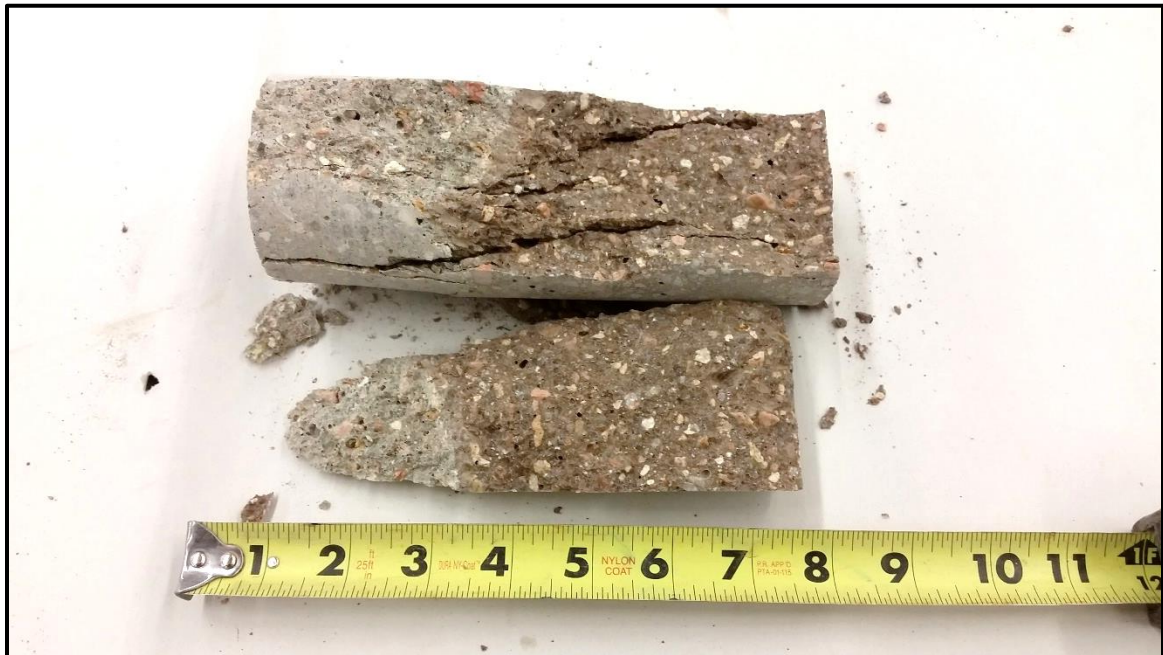
Figure 3-20 – Same specimen as Figure 3-19, opened to reveal surface of splitting tension failure. Note colored concrete is overlay; gray concrete is substrate
