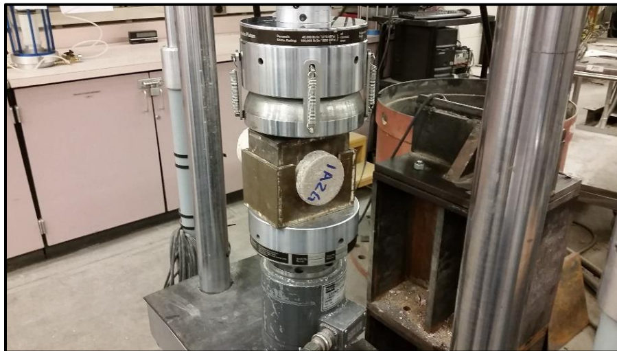
Figure 2-2 – Direct shear test in-progress
