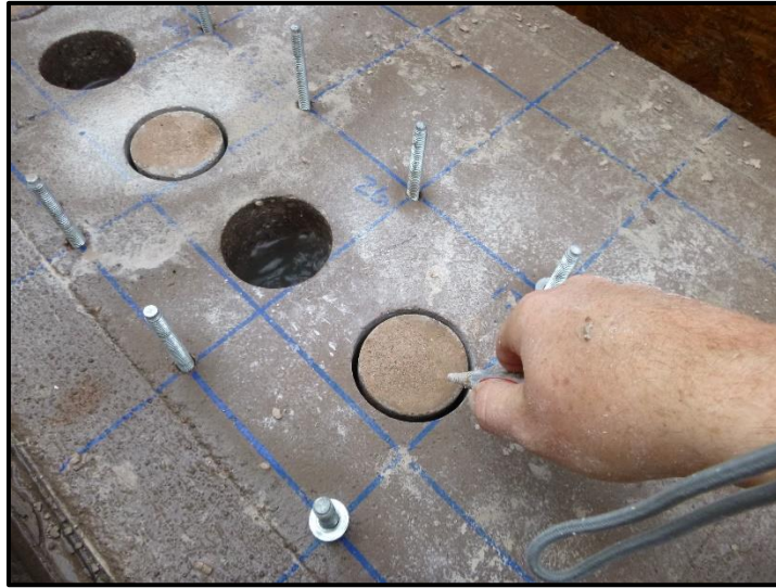
Figure 3-12 – Cleaning the surface of the pull-off test specimen
