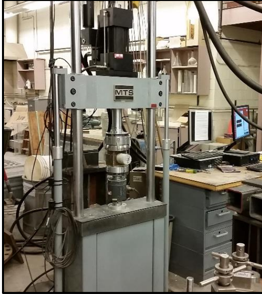
Figure 3-14 – MTS testing equipment with direct shear apparatus
