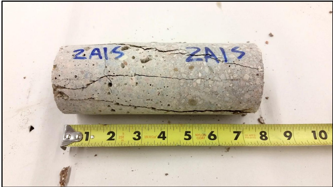
Figure 3-19 – Representative slant shear cylinder after testing under uniaxial compression
